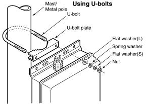
**WARNING:** Mount the AT-140 securely with the supplied nuts and bolts. Otherwise, vibrations and shocks due to waves, etc. could loosen the antenna tuner making if fall, causing personal injury.
