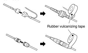
3 Fix both of the coaxial and control cables to protect the inside connections.
